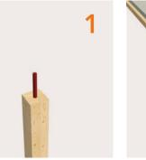
The facade column is put into position, with a steel connector ready fitted
