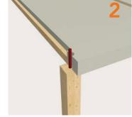
The slab elements are fitted (timber-concrete composite)
