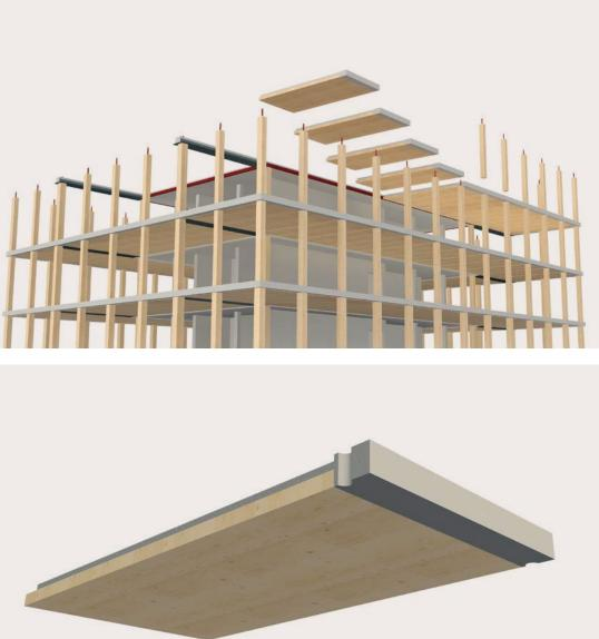
The following illustrations show how the individual prefabricated parts are joined together to form a stable unit.
